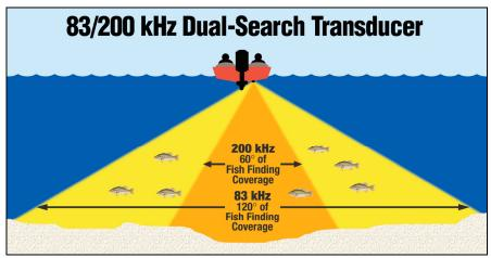
A new innovation, the 83 kHz frequency offers superior sonar performance at all depths from very shallow up to 1,000 ft and provides up to 120° of fishfinding coverage.
